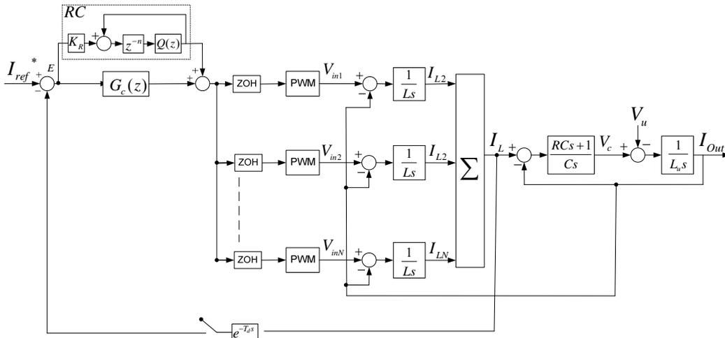
Fig. 2. Overall single-phase block diagram of the interleaved grid connected inverter and its controller
