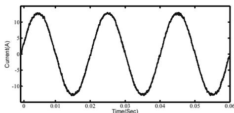
Fig. 13. Simulated output current with RC (THD=2.2%)
