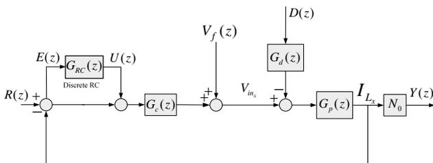
Fig. 3. The simplified general diagram of the system with proposed control scheme
