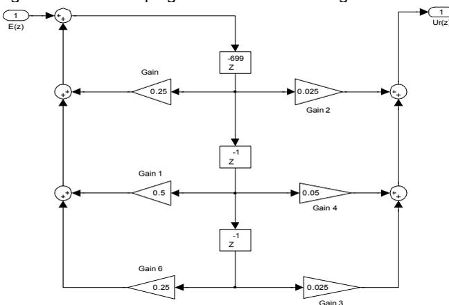
Fig. 11. Implementation of RC in direct form II
