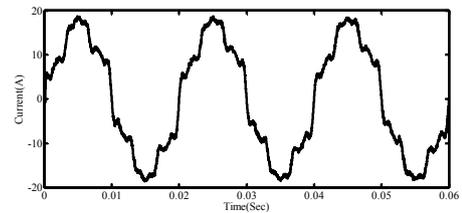
Fig. 14. Simulated output current without RC (THD=22%)
