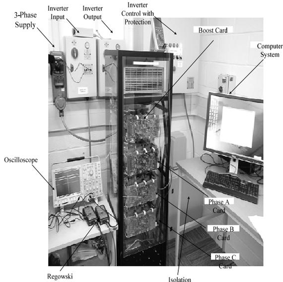
Fig. 8. Experimental test rig of the three-phase interleaved inverter
