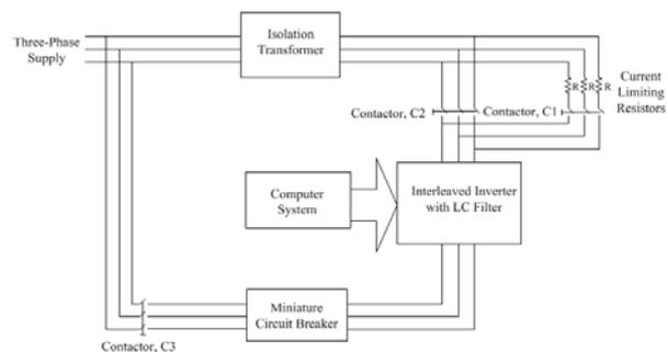
Fig. 7. Schematic diagram of the power circuit of the experimental apparatus
