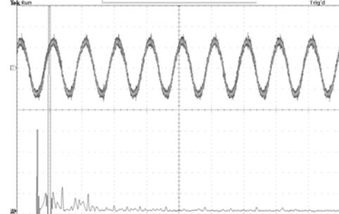
Fig. 15. Output current using RC (THD=2.0%)
