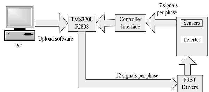
Fig. 6. Basic hardware configuration for single-phase
