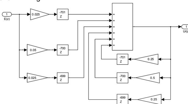
Fig. 10. Implementation of the RC in direct form I
