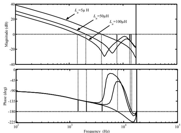
Fig. 4. Bode plot of the system with conventional tracking controller  $G_c(z)$  against grid impedance variations
