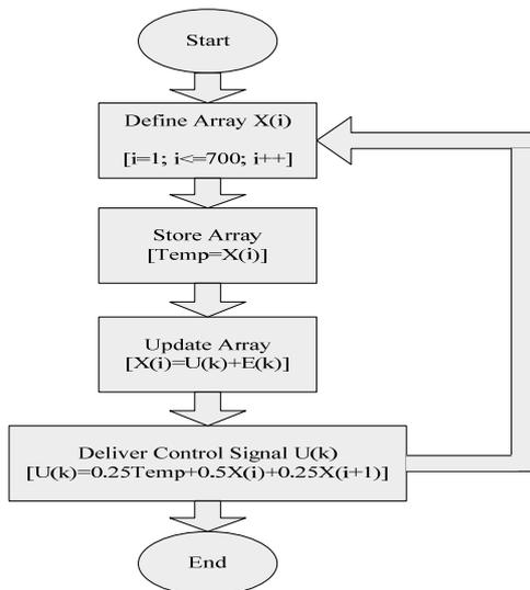
Fig. 12. Flowchart of the algorithm for implementation of the RC
