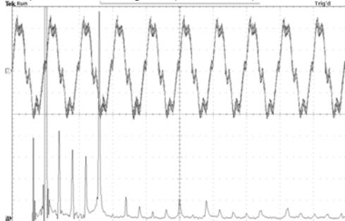
Fig. 16. Output current without RC (THD=16%)
