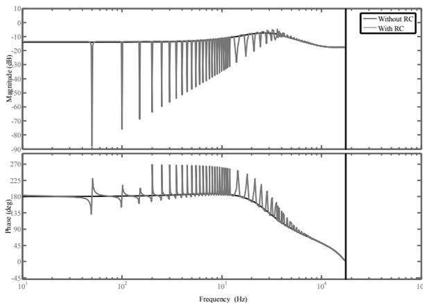
Fig. 5. Frequency response of the disturbance transfer function
