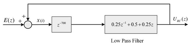
Fig. 9. Elements of the RC when  $K_R = 1$  and  $G_f(z) = 1$
