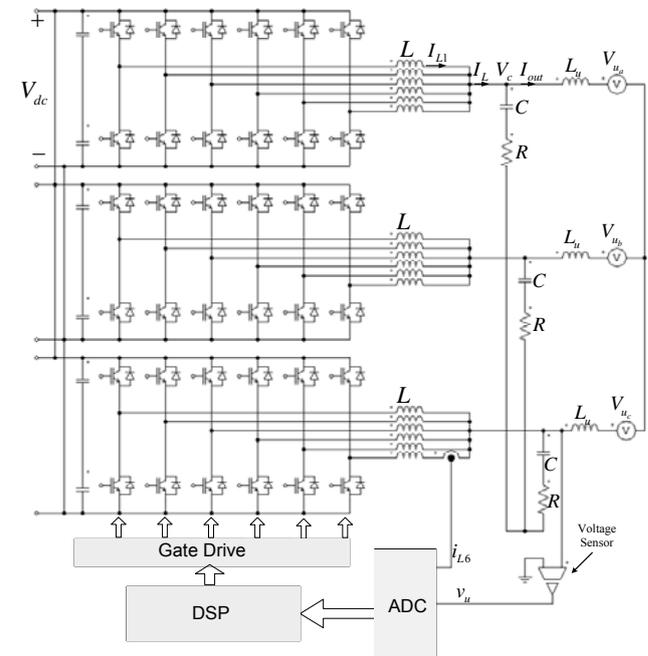
Fig. 1. Three-phase interleaved grid connected inverter-showing control of one channel of single phase
