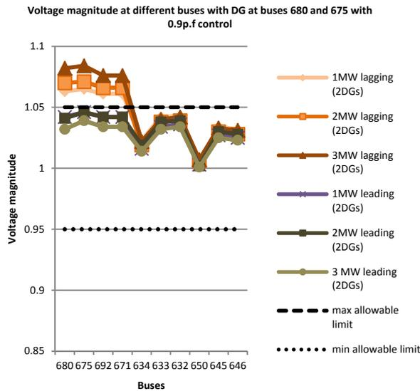
Fig. 2: Voltage magnitude at different buses with DG operating at 0.90 p.f.
