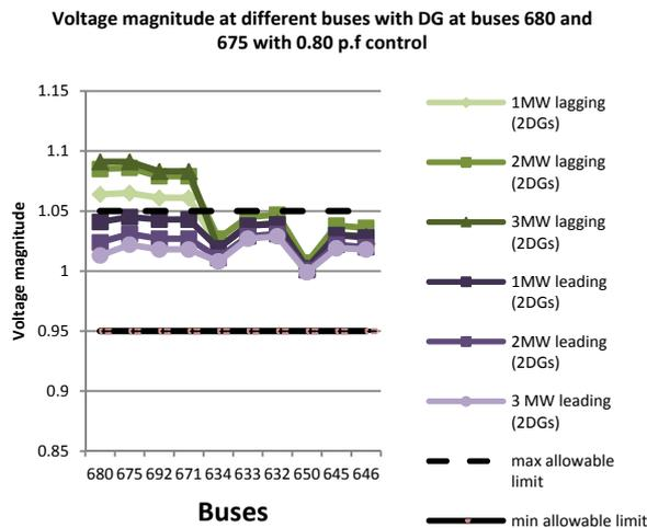
Fig. 3: Voltage magnitude at different buses with DG operating at 0.80 p.f.
