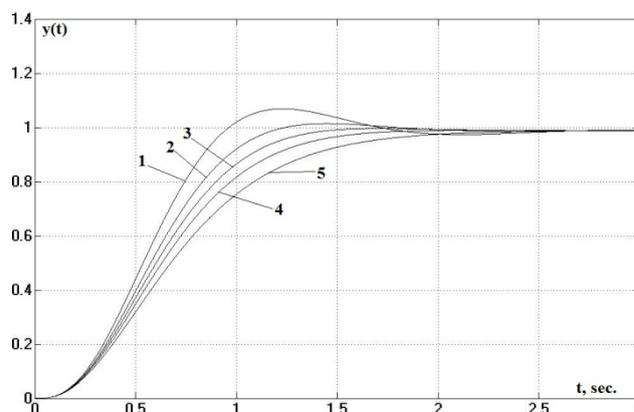
Fig. 1. Output signal of the system in the case of configuration to 1) standard form of Butterworth; 2)  $\lambda_1 = 0.7$ ; 3)  $\lambda_1 = 0.5$ ; 4)  $\lambda_1 = 0.3$ ; 5) binomial form.
