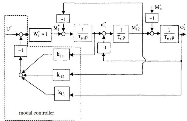
Fig. 3. The scheme of modal speed control
