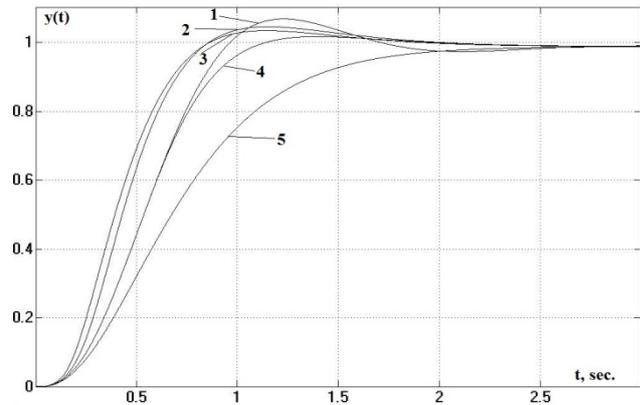
Fig.4 Output signal of the system in the case of configuration to 1) standard form of Butterworth; 2) subsystem with one root in the right half-plane  $L(u; 0.87, 0.88)$ ; 3) subsystem with two roots in the right half-plane  $L(u; 0.9, 0.96)$ ; 4) stable subsystems synthesized according to standard forms of Butterworth and binomial  $L(u; 0.48, 0.5)$ ; 5) binomial form
