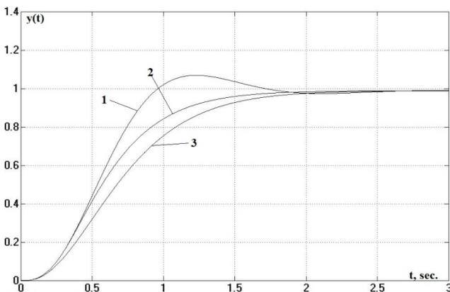
Fig. 2. Output signal of the system in the case of configuration to 1) standard form of Butterworth; 2)  $\lambda_1 = 1 - \lambda_2 = L(x_{inp} - x(t); 0.8, 0.9)$  sec.; 3) binomial form
