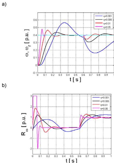
Fig. 5. Influence of the  $\eta$  coefficient of the speed controller to the speed transient (a) and the output signal of the speed controller (b).
