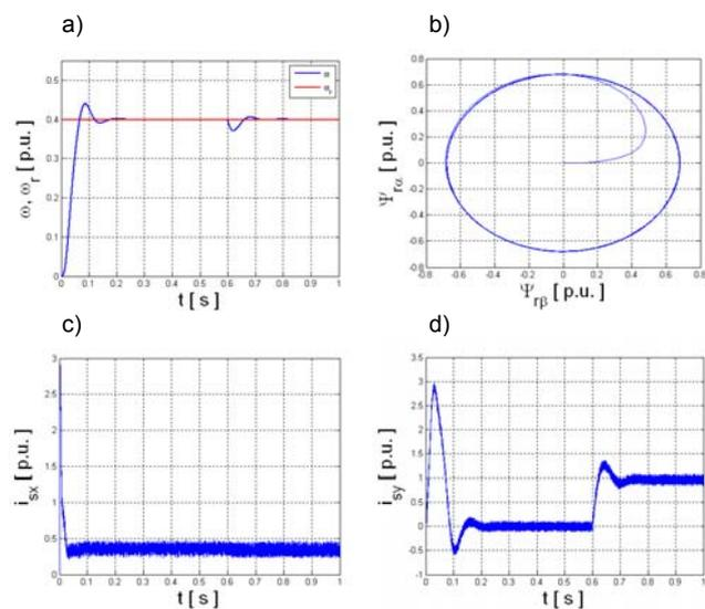
Fig. 3. Transients of state variables in analyzed drive: the actual and reference speed (a), hodograph of the rotor flux (b), components of the stator current vector (c, d)
