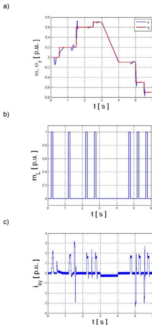
Fig. 4. Transients of the drive and reference speed (a), load torque changes (b) and  $i_{sy}$  component of the stator current (c)
