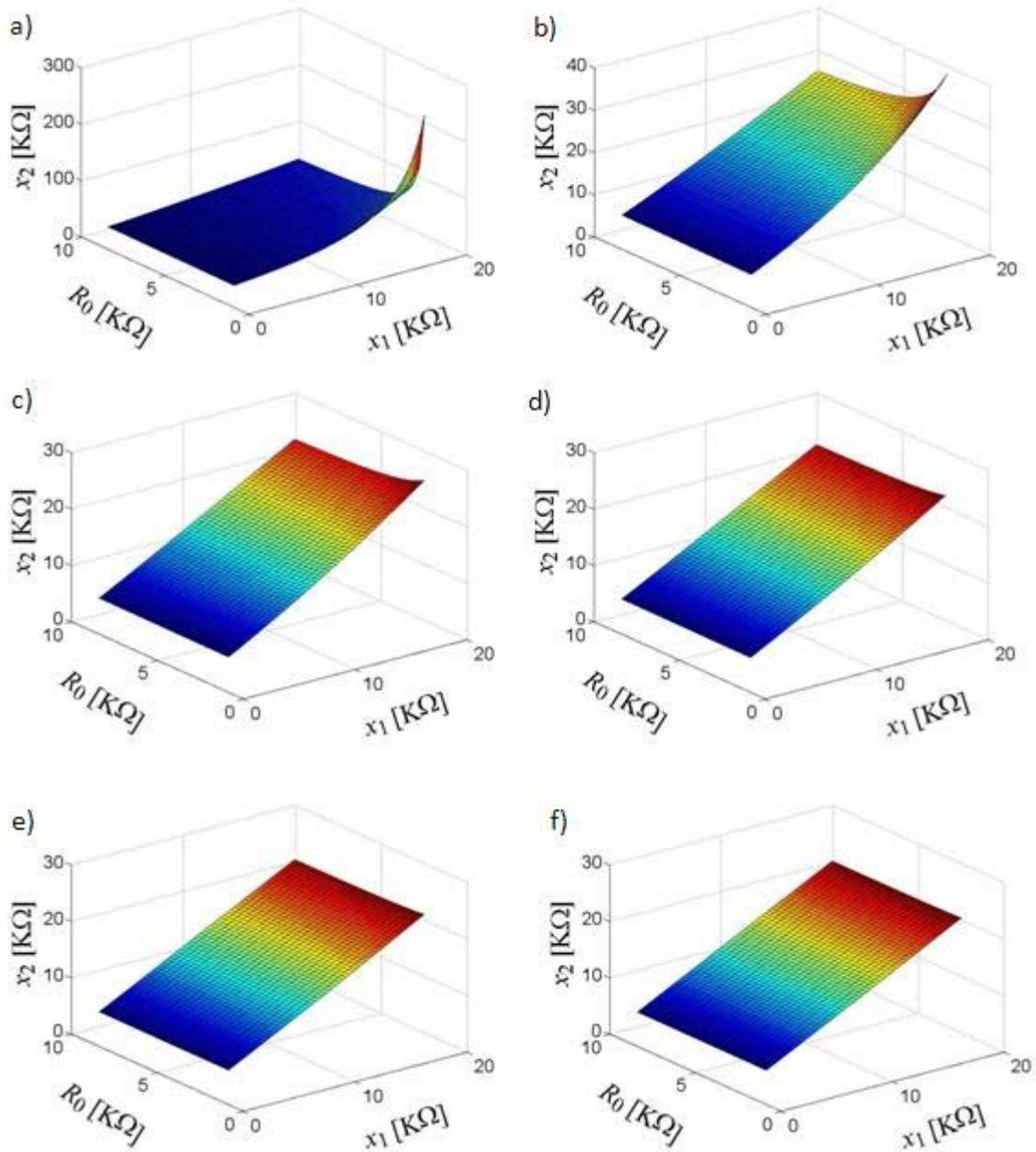
Fig.5. Simulation results for the measurement model of the circuit with different precisions. a)  $k=10\%$ , b)  $k=5\%$ , c)  $k=2\%$ , d)  $k=1\%$ , e)  $k=0.5\%$ , f)  $k=0.2\%$
