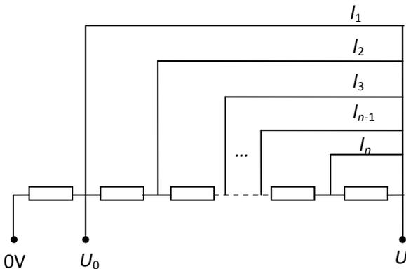
Fig.3. Inner circuit of the designed sensor
