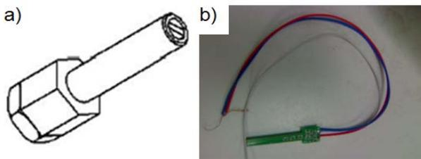
Fig.2. Designed sensor. a) appearance of the sensor, b) electronic chip inside the sensor
