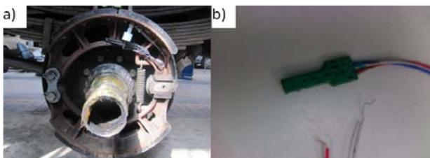
Fig.6. Experiments on a brake shoe with the designed sensor. a) installation of the sensor, b) worn electronic chip inside the sensor
