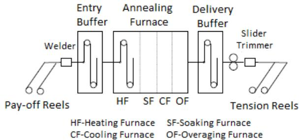
Fig.3. Outline of a continuous annealing process [13]
