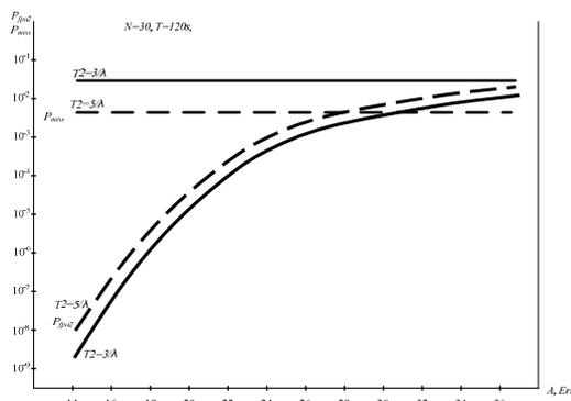
Fig. 8. Decreasing of false pre-alarm probability may be obtained by increasing of probability of miss (two-step detector)
