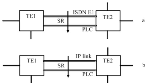
Fig. 1. Model of two network nodes connected by ISDN (a) or IP (b) link and PLC
