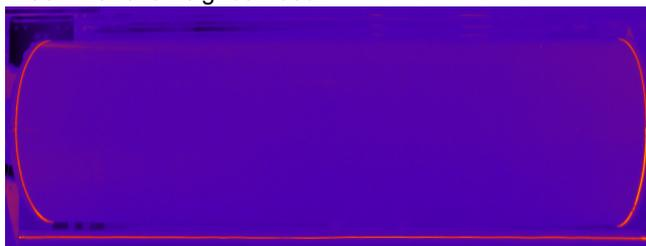
Fig.2. Hot markers illustrate outlines of the cylinder and the horizontal marker for camera roll angle correction
