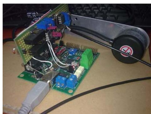
Fig.3. Electronic synchronization module with for IR camera
