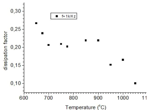
Fig.3 The dissipation factor of the coal ash sample heated at temperatures in the range of  $600\text{ }^\circ\text{C}$  +  $1100\text{ }^\circ\text{C}$
