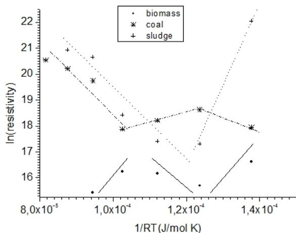
Fig.2. The resistivity of the sewage sludge ash, coal ash and biomass ash sample heated at temperatures in the range of  $500\text{ }^\circ\text{C}$  +  $1100\text{ }^\circ\text{C}$
