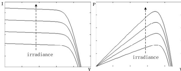
Fig.3 Output characteristics of PV module under different irradiance
