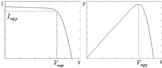
Fig.2 Output characteristics of PV cel
