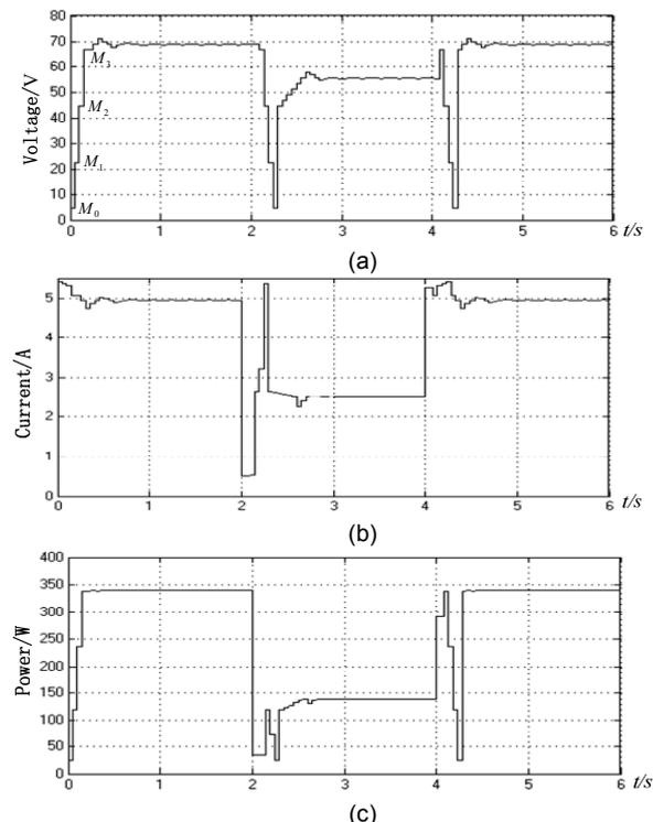
Fig.9 The working process of GMPPT controller (a) Output voltage; (b) Output current; (c) Output power
