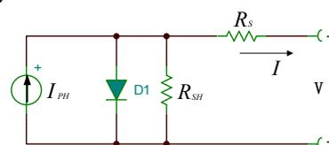
Fig.1 Equivalent circuit model of PV cell
