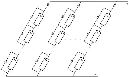
Fig.6 Series-parallel(SP) solar PV array
