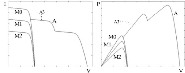
Fig.5 Output characteristics of 3 PV modules and their series connection under different irradiance
