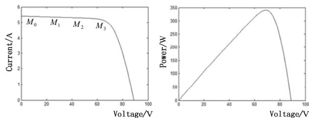
Fig.7 Output curves of the PV array under uniform irradiance
