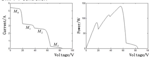
Fig.8 Output curves of the PV array under PSCs
