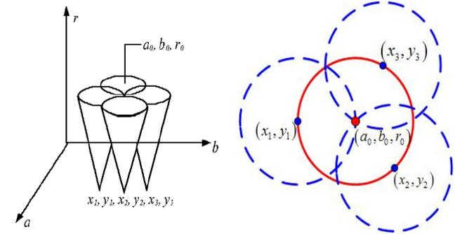
Fig.3. Hough transform and circle detection
