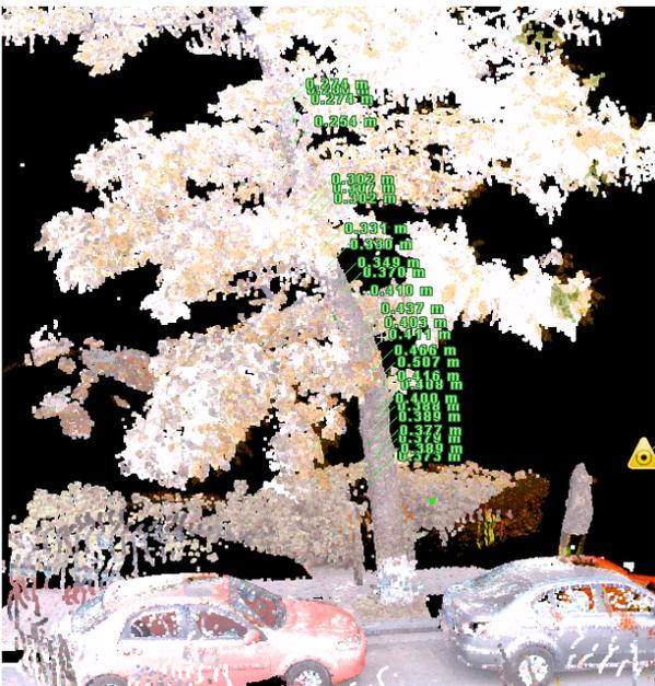
(a) Manually extract main stem diameter from leica cyclone point data
