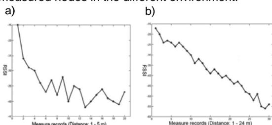
Fig.5. a) The RSSI varying from 1m to 5m indoors
