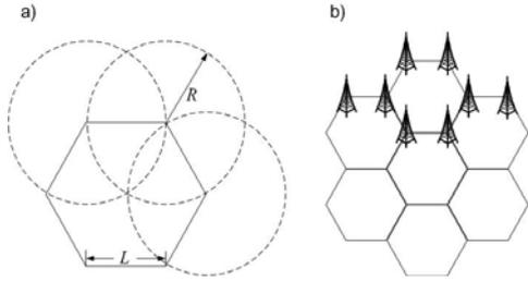
Fig.1. a) Each hexagon like deployment of the base station b) Cellular deployment made up by hexagons
