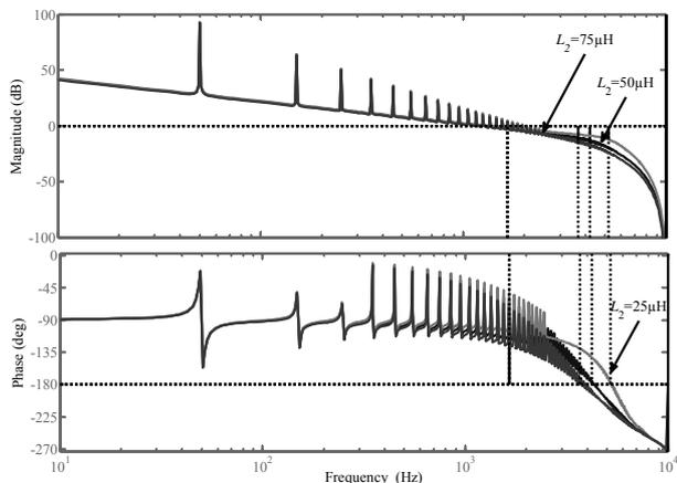
Fig.7. Effect of variations in  $L_2$  on the ORC system
