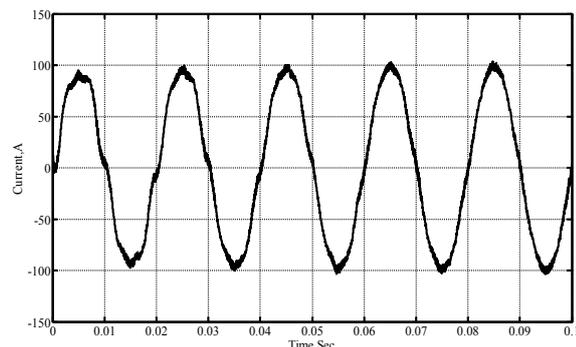
Fig.6. Output current with ORC
