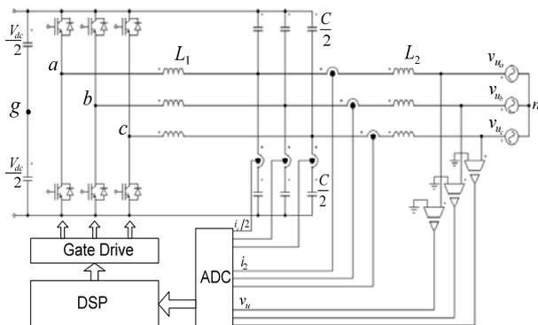
Fig. 1: Two-level grid connected inverter with LCL filter
