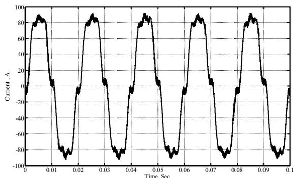
Fig.5. Output current without ORC
