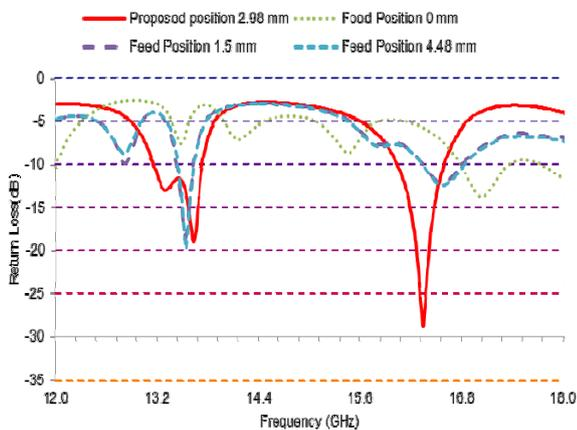
Fig. 5 S<sub>11</sub> with different feed position
