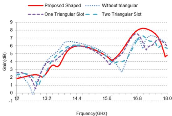
Fig. 4. Simulated Gain of four types of antenna
