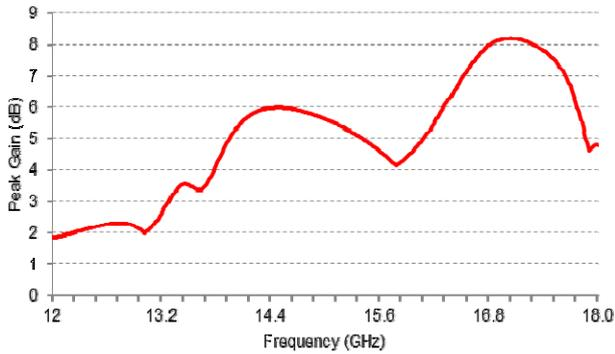
Fig 7. Peak Gain of the proposed shaped
