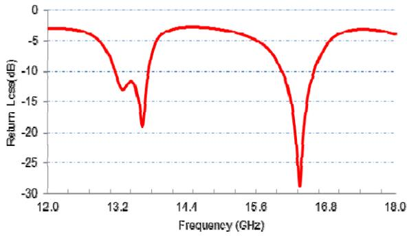
Fig. 6. Return loss of the proposed shape
