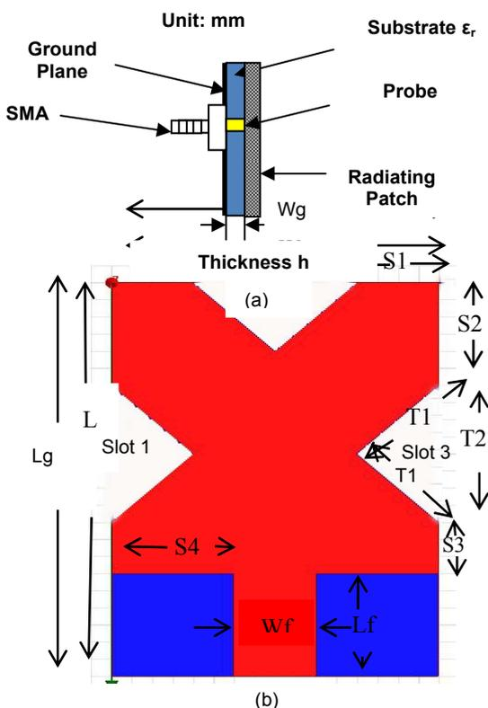
Fig. 1: Configuration of the proposed patch antenna (a) Side view (b) Top View
