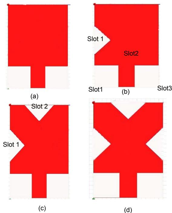
Fig. 2: Geometry of a) Without slot antenna b) one equilateral triangular slot antenna c) Two equilateral triangular slot antenna d) Proposed shape antenna
