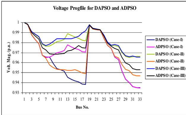
Fig. 6. IEEE 33-bus radial distribution system bus voltage for DAPSO and ADPSO in Case-I, Case-II and Case-III
