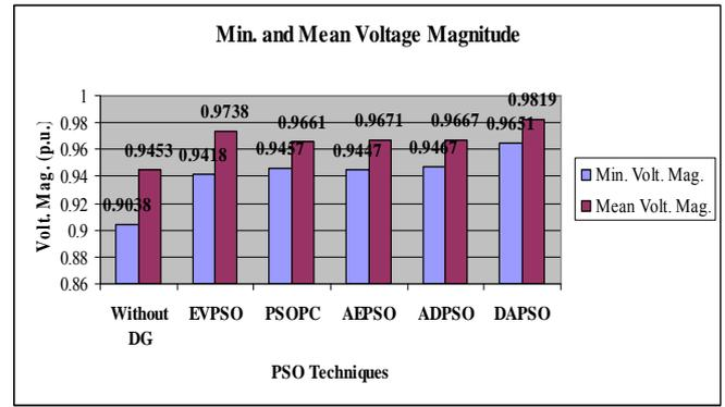
Fig. 5. Min. and mean voltage values for different PSO techniques in Case-II
