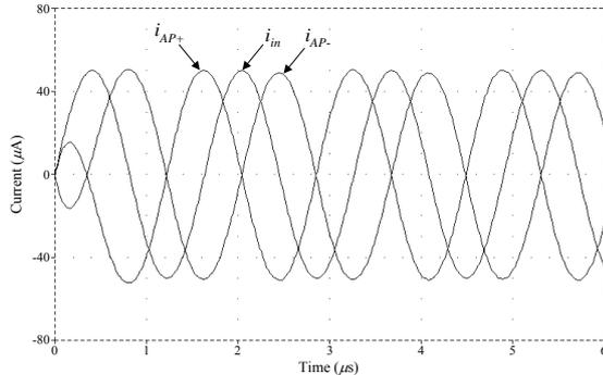
Fig.6 Time-domain responses of the proposed AP filter for input frequency 612 kHz.
