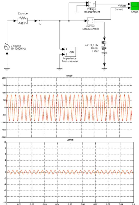
Fig.3. Measuring scheme with voltage source whose parameters are: ideal sinusoidal AC voltage, amplitude 100V; phase position (0):0; frequency (Hz):10-104; initial time-0 source impedance  $Z_{source}$  parallel link R1L,  $R(\Omega)=10$ ;  $L(H)=10e-03$ , RLC - parameters filter: resistance  $R(\Omega)=1$ ; inductivity  $L(H)=1e-03$ , capacitance  $C(F)=1e-06$
