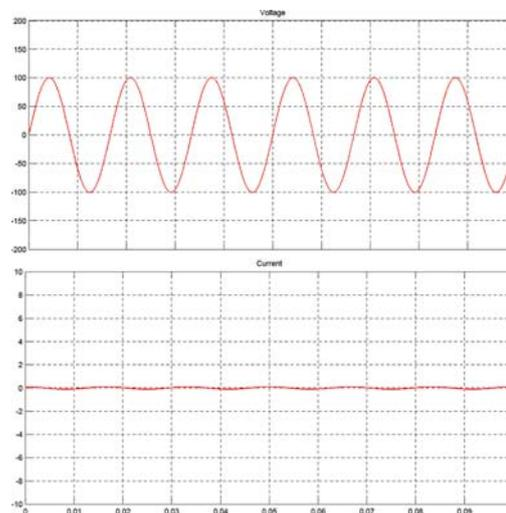
Fig.7. Basic harmonic of voltage and current measured by linear filter with serial  $RC$  impedance [ $R(\Omega)=1$ ;  $C(F)=10e-06$ ], ans diagrams: voltage ordinate  $\pm 200V$ , current ordinate  $\pm 10A$ ,  $f=50Hz$
