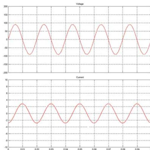
Fig.6. Basic harmonic of voltage and current measured by linear filter with serial  $RL$  impedance  $R(\Omega)=1$ ;  $L(H)=100e-03$ , diagrams: voltage ordinate  $\pm 200V$ , current ordinate  $\pm 10A$ ,  $f=50Hz$
