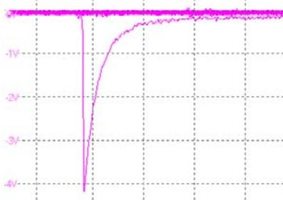
Fig.9. Measured curve of depolarization current
