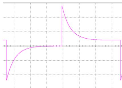
Fig.5. Simulation of PDC with extended Debye model.
