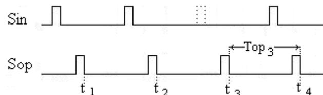
Fig. 3 The lost pulse is recovered;  $T_{op3}$  is increased for  $t_c$
