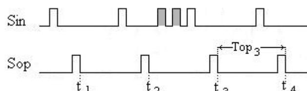
Fig. 4 Black pulses are eliminated;  $T_{op3}$  is decreased for two  $t_c$
