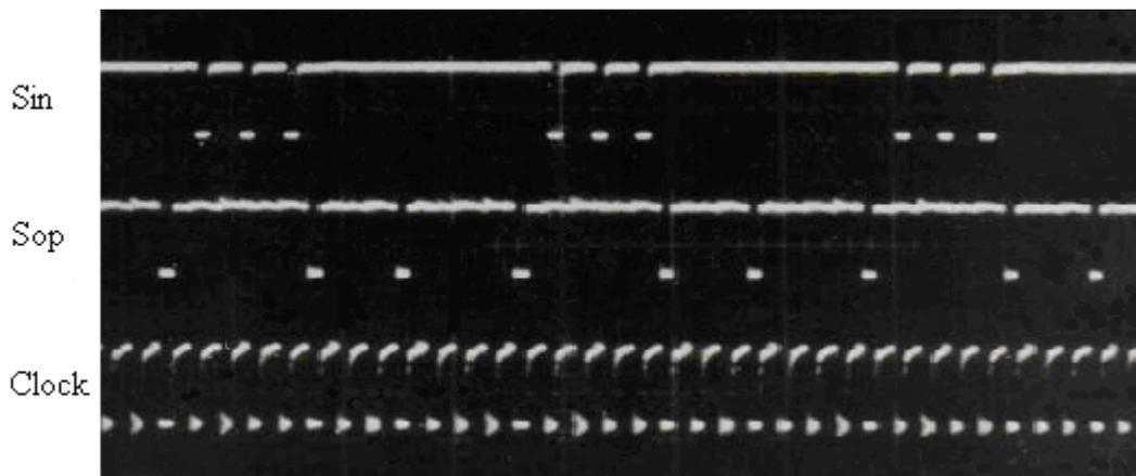
Fig. 5 Timing diagram of the FLL signals; the functioning of FLL may be followed in real time for every pulse
