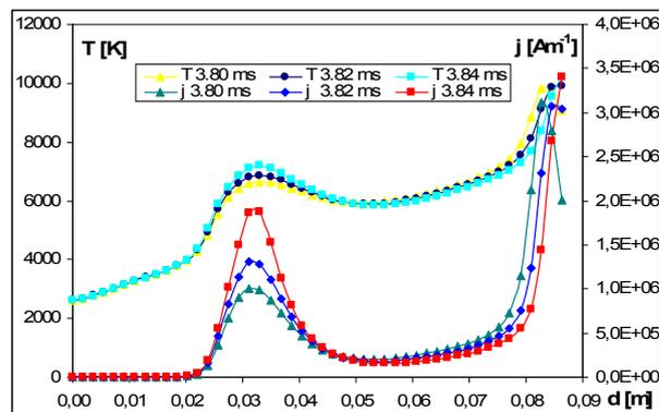
Fig. 7. Temperature and current density distribution on the electrode arrangement model axis at time intervals from 3.80 ms to 3.84 ms
