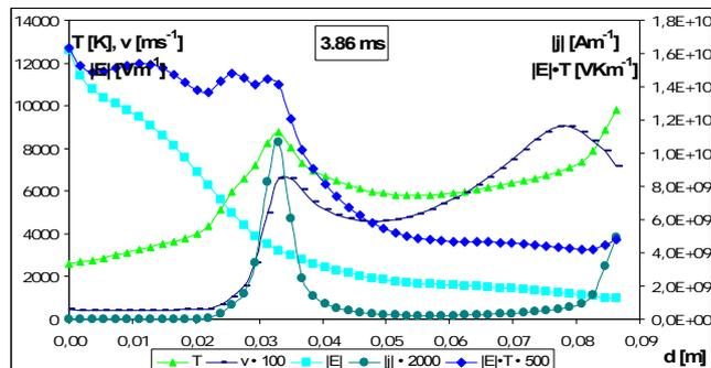
Fig. 10. Temperature T, mass velocity v, strength of the electric field E, current density distribution j, strength of the electric field and temperature product  $|E| \cdot T$  on the electrode arrangement model axis at the time point of 3.86 ms
