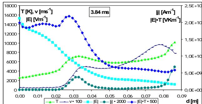
Fig. 9. Temperature T, mass velocity v, strength of the electric field E, current density distribution j, strength of the electric field and temperature product  $|E| \cdot T$  on the electrode arrangement model axis at the time point of 3.84 ms
