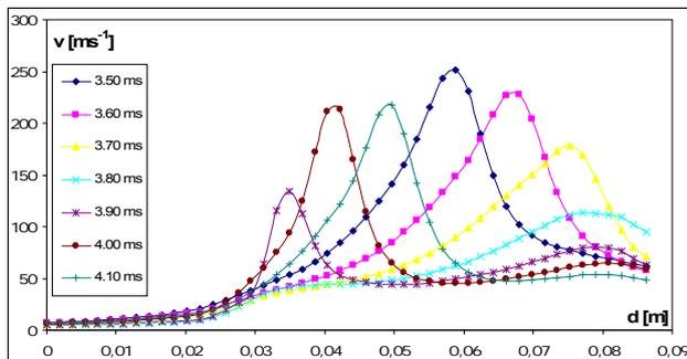
Fig. 4. Mass velocity distribution on the electrode arrangement model axis at time intervals from 3.50 ms to 4.10 ms
