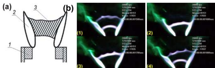
Figure 1. Contacts 1 with plasma streams 2 and a discharge channel 3, connecting the plasma streams: a) Diagram; b) Subsequent frames 1÷4 in a model system (exposure time of 50  $\mu$ s, 100  $\mu$ s interval) illustrating the formation of a new discharge channel between the plasma streams
