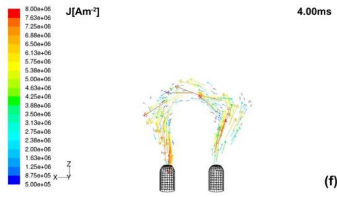
Fig. 3. Selected frames of computer simulation of an AC electric arc burning freely in the air at  $I_{max} = 500A$ , at atmospheric pressure, during one current half-period. Temperature distributions are shown on the left side (a,b,c) and the corresponding pictures of current density vectors (d,e,f) at times  $t=3.85$  ms,  $t=3.90$  ms and  $t = 4.00$  ms are shown on the right side, respectively
