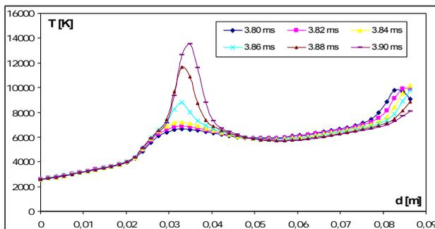
Fig. 6. Temperature distribution on the electrode arrangement model axis at time intervals from 3.80 ms to 3.90 ms
