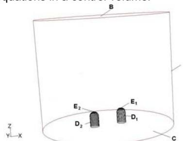
Fig. 2. The modeled arrangement of parallel electrodes. A, B, C – surfaces determining the limit surfaces; E<sub>1</sub>, E<sub>2</sub> – the surfaces of electrode tips, D<sub>1</sub>, D<sub>2</sub> – the lateral surfaces of the electrodes
