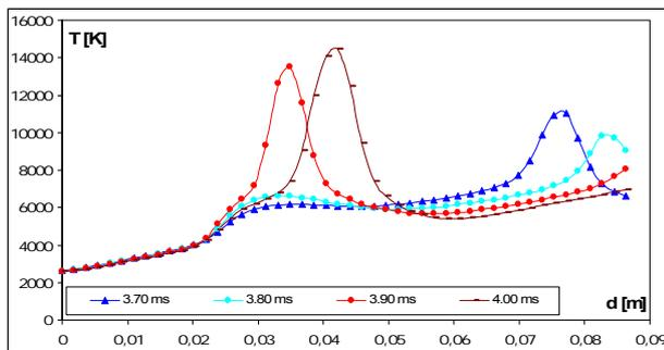
Fig. 5. Temperature distribution on the electrode arrangement model axis at time intervals from 3.70 ms to 4.00 ms.
