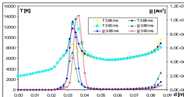
Fig. 8. Temperature and current density distribution on the electrode arrangement model axis at time intervals from 3.86 ms to 3.90 ms
