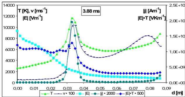
Fig. 11. Temperature  $T$ , mass velocity  $v$ , strength of the electric field  $E$ , current density distribution  $j$ , strength of the electric field and temperature product  $|E| \cdot T$  on the electrode arrangement model axis at the time point of 3.88 ms
