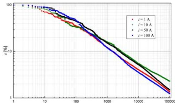
Fig. 5. The boundary error versus number of iterations for various exciting current values
