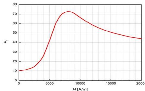
Fig. 4.  $\mu(H)$  dependence (steel ST35)
