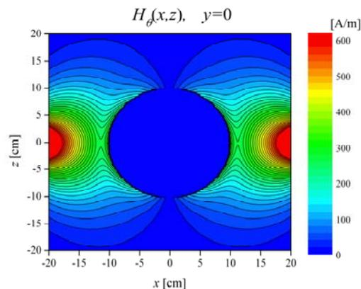
Fig. 8. Computed distribution for the zenith component of the magnetic field intensity
