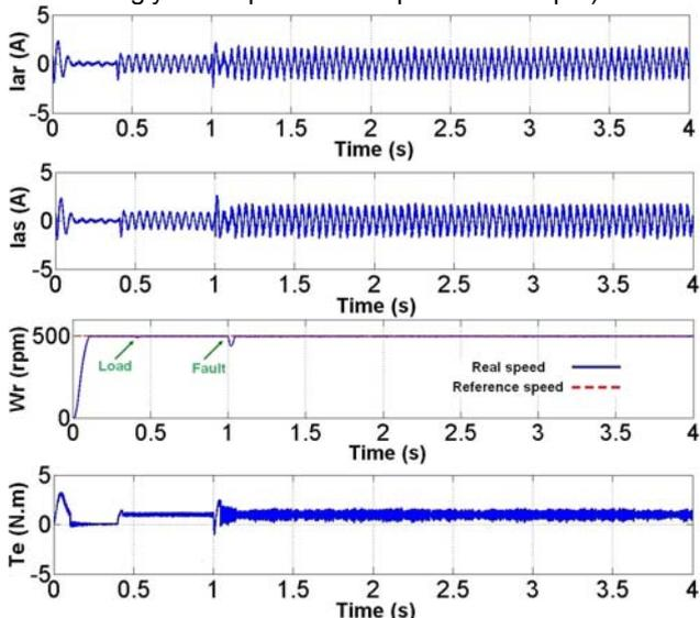
Fig.5. Simulation results of the proposed modified controller (Rotor a-axis current, Stator a-axis current, Rotor speed, Electromagnetic torque)
