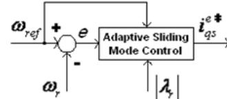
Fig.3. Scheme of the speed controller with adaptive sliding mode
