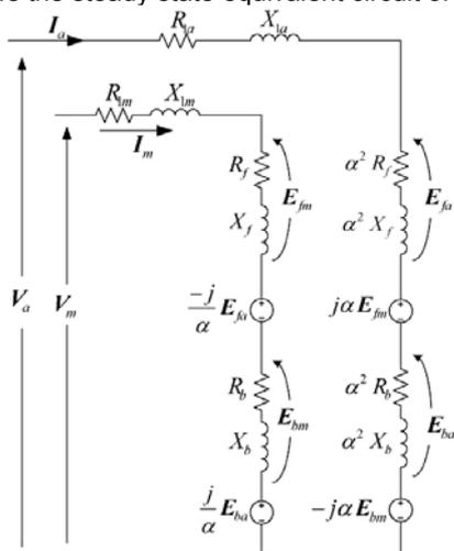
Fig.1. Steady state equivalent circuit of SPIM
