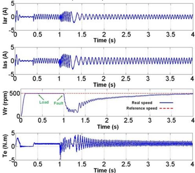
Fig.4. Simulation results of the conventional controller (Rotor a-axis current, Stator a-axis current, Rotor speed, Electromagnetic torque)
