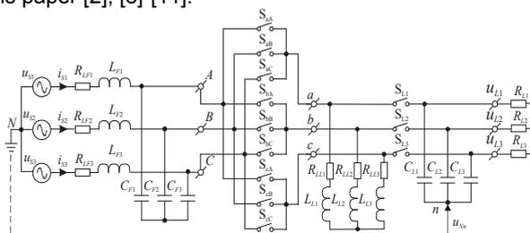
Fig. 1. Topology of Matrix-Reactance Frequency Converter based on matrix reactance chopper with buck-boost topology
