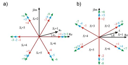
Fig. 3. Graphical interpretation of: a) sectors of the output voltage vectors, b) sectors of the input line current vectors
