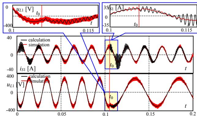
Fig. 5. Transient responses of input current and output voltage at step change of  $f_L$  from 50 to 20 Hz,  $D_S=0.6$
