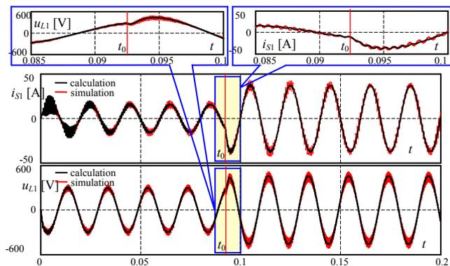
Fig. 4. Transient responses of input current and output voltage at step change of  $D_S$  from 0.5 to 0.75,  $f_L=25\text{Hz}$
