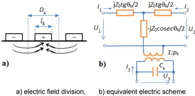
a) electric field division, b) equivalent electric scheme
