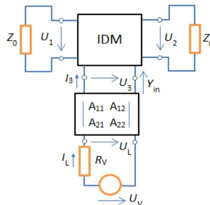
Fig.4. IDT equivalent scheme model on triple gate basis with optional double gate matching circuit
