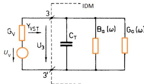
Fig.5. IDT equivalent scheme
