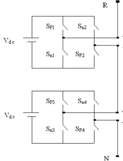
Fig.3. One-leg circuit of five-phase five-level CHMLI
