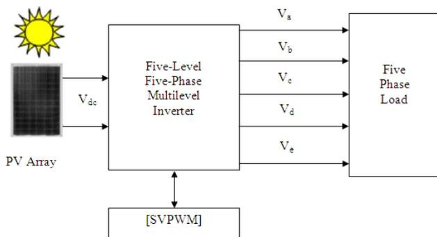
Fig.1. General diagram of the proposed system
