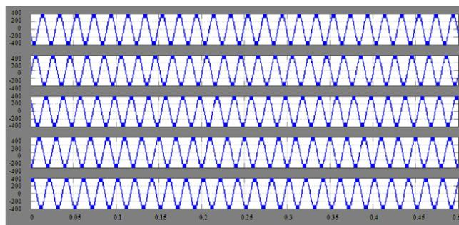
(a) Line-to-Line voltage of a five-phase five-level DCMLI
