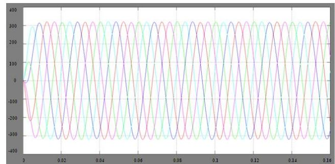
(a) Line-to-Line voltage of a five-phase five-level CHMLI
