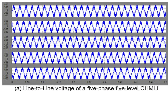
(a) Line-to-Line voltage of a five-phase five-level CHMLI
