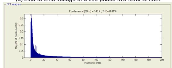
(b) THD measurement of a proposed five-phase five-level CHMLI
