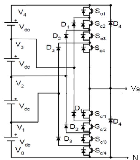
Fig.4. One-leg circuit of five-phase five-level DCMLI
