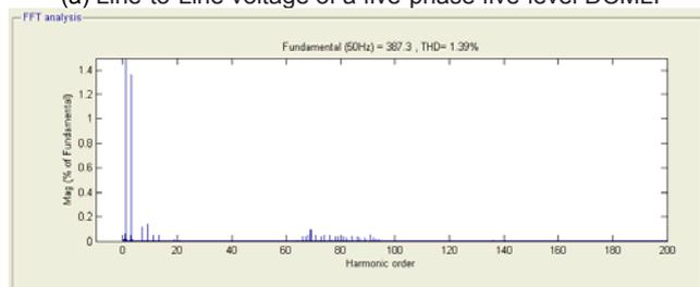
(b) THD measurement of a five-phase five-level DCMLI
