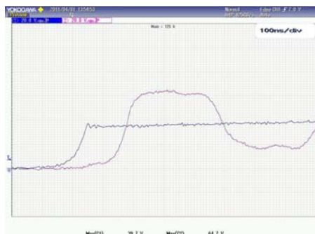
Fig.5. Oscillograms of voltage: CH1 voltage on the SPD terminals ( U_p = 40 V), CH2 voltage at apparatus to be protected, represented by resistive load, R = 1 M \Omega ; Stressing impulse voltage wave shape 1,2/50 \mu s ; connecting leads length d = 30 m
