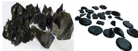
Fig.3. The products of the immersed arc treatment of contaminated minerals [22]. The crashed frozen lava like and cake like casts
