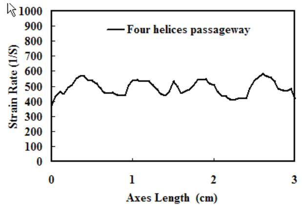
(b) Strain rate in axial direction
