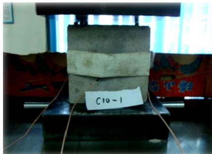
Fig. 7. The concrete sample of this uniaxial compression test
