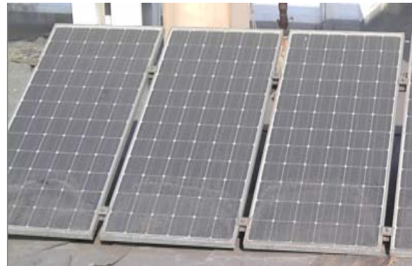
Fig.6. Naturally polluted PV module and different dust thickness
