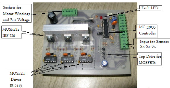
Fig.4. Driving card of the BLDC motor with its all equipments.
