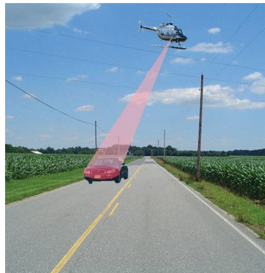
Fig. 3. The HPM uses microwave energy to disable or damage vehicle electronic control modules/microprocessors that control vital functions of engines. Image courtesy of Defense Intelligence Agency (DIA).
