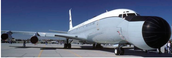
Fig. 8. Modified C-18A (converted Boeing 707) as EC-18B advanced range instrumentation aircraft (ARIA) with 2.1-m diameter radar dish on the nose.
