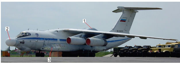
Fig. 5. Russian Beriev A-60 (modified IL-76MD) with HEL turret and nose mounted radar. 1.1-MW HEL turret, 2 — radar for detecting aerial targets, 3 — compartment for 2.1 MW turboalternator. Photograph taken at Taganrog Yuznyi Airport in May 2011 by O. Ziminov, RovSpotters Team.
