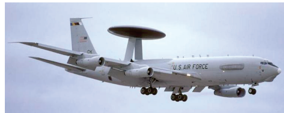
Fig. 7. AR mounted in rotodome on E-3B Sentry (Boeing 707 adapted to military functions).
