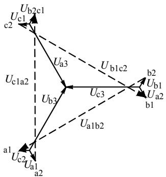
Fig.7. Phasor diagrams of  $Yd_6y_6$  transformer secondary voltages; a) modified delta winding voltages, b) modified wye winding voltages. Phase voltages are marked with continuous lines; dashed lines denote maximum potential differences between individual phase terminals ("undesirable" or "incorrect" voltages)
