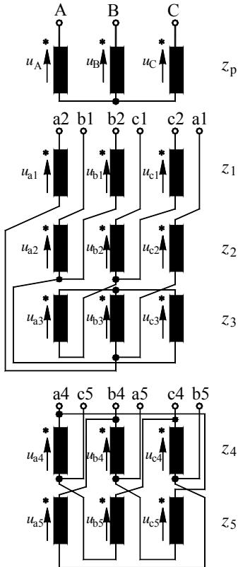
Fig.5. Transformer designated as  $Yd_6y_6$  - windings scheme
