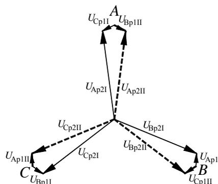
Fig.3. Transformer denoted as 2(Y<sub>2</sub>yd) - phasor diagram of primary voltages
