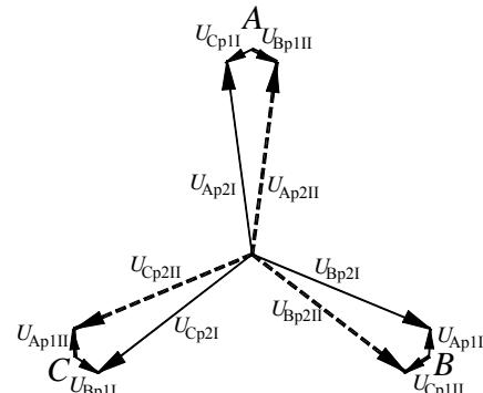
Fig.3. Transformer denoted as 2(Yzd) - phasor diagram of primary voltages
