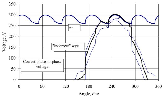
Fig. 10. Transformer-rectifier operation, system loaded, rectifiers connected in parallel; modified wye winding voltage waveform, thick black line marks voltage between potentials belonging to different phases, thinner lines show correct phase-to-phase voltages; rectified voltage waveform  $u_0$  is also shown
