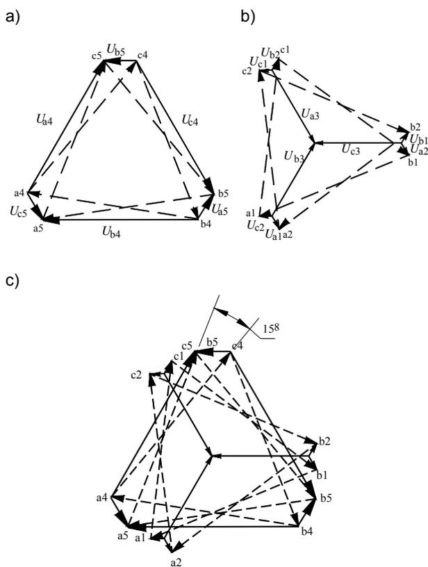
Fig.6. Phasor diagram of secondary voltages,  $Yd_6y_6$  transformer; a) modified delta winding, b) modified wye winding, c) all phase and phase-to-phase voltages. Phase-to-phase voltages marked with dashed lines. Voltage designations as in Fig.5
