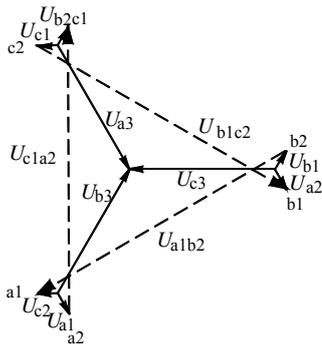
Fig. 7. Phasor diagrams of Yd<sub>6</sub>y<sub>6</sub> transformer secondary voltages; a) modified delta winding voltages, b) modified wye winding voltages. Phase voltages are marked with continuous lines; dashed lines denote maximum potential differences between individual phase terminals (“undesirable” or “incorrect” voltages)
