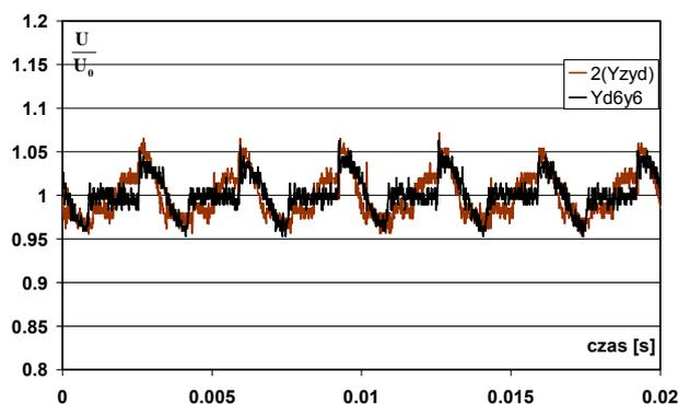
Fig.13. Rectified voltage waveforms (additional waveforms given for 2(Yzyd) transformer) - rectifiers connected in parallel
