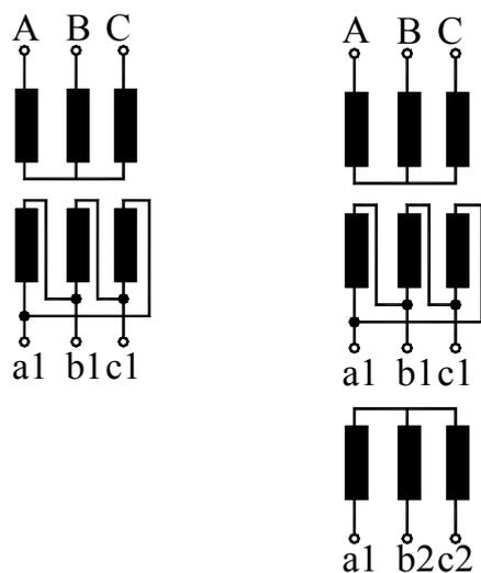
Fig.1. Rectifier 3-phase (Yd) and 6-phase (Yyd) transformer - windings schemes
