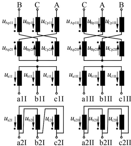
Fig.4. Transformer denoted as 2(Y<sub>2</sub>yd) - windings scheme
