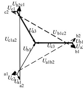
Fig. 8. Transformer-rectifier operation, very small load, rectifiers connected in parallel; a) modified wye winding voltage waveforms, b) current path, modified wye winding and corresponding bridges shown only, c) voltage acting in this circuit  $U_{b1c2}$  (marked with dashed line on modified wye phasor diagram)
