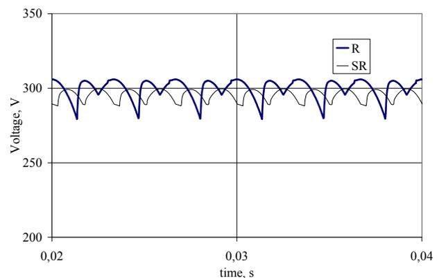
Fig. 12. Rectified voltage waveform, no-load operation, rectifiers connected in parallel (R) and series-parallel (SR)
