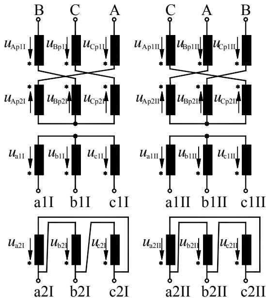
Fig.4. Transformer denoted as 2(YzYd) - windings scheme
