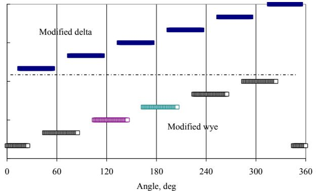
Fig. 9. Changeover of voltages in the circuit (unloaded): lower half of drawing relates to “incorrect” voltages from modified wye system, upper half relates to “incorrect” voltages from modified delta system (cf. Fig. 7)
