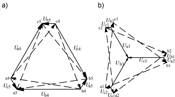
Fig.6. Phasor diagram of secondary voltages,  $Yd_6y_6$  transformer; a) modified delta winding, b) modified wye winding, c) all phase and phase-to-phase voltages. Phase-to-phase voltages marked with dashed lines. Voltage designations as in Fig.5
