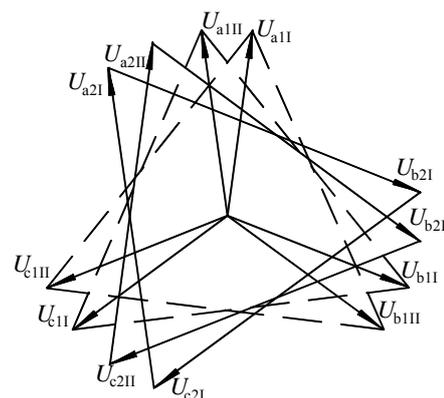
Fig.2. Phasor diagram of secondary voltages of 12-phase transforming circuit consisting of two Yyd transformers; windings marked as in Fig.3; dashed line marks phase-to-phase voltages of wye-connected windings
