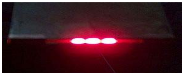
Fig.5. Waveguide slit neon plasma for absorbed microwave power P_A=65 W. Gas flow rate Q=25 l/min.
