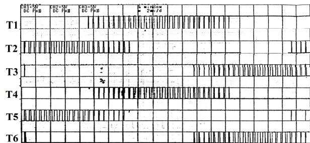
Fig.6 Experimental waveforms of the three complementary pairs of inverter drive signals
