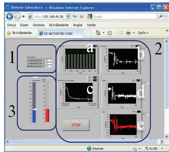
Fig. 4. Front panel of PID control application of a DC motor
