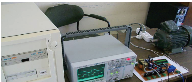
Fig.7. The designed cosφ meter experimental setup
