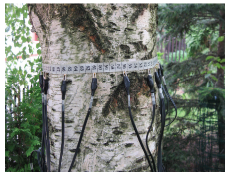
Fig. 6. The measurement stand during the tomography testing of the birch
