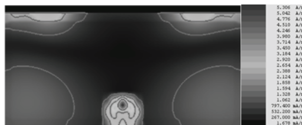
Fig. 7. ACD @ 140kHz – vertical cross section of the phantom.
