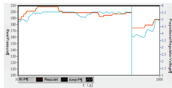
Fig.5. Controlled common-rail pressure curve at aimed value of 200 MPa
