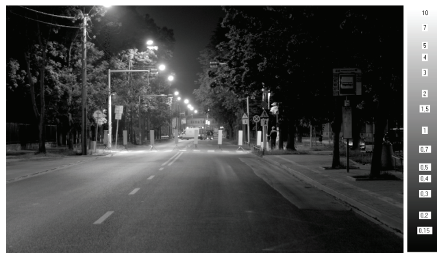
Fig. 7. Luminance measurement for targets of the first observation direction (logarithmic scale \log_2 , unit \text{cd}/\text{m}^2 )
