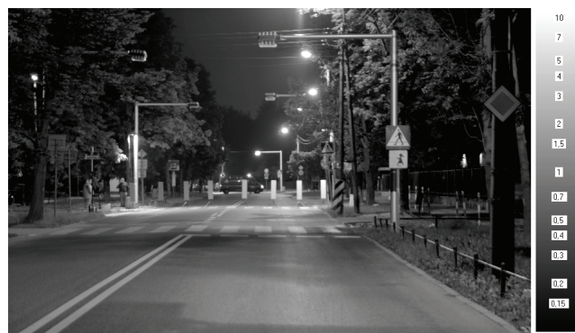
Fig. 8. Luminance measurement for targets of the second observation direction (logarithmic scale \log_2 , unit \text{cd}/\text{m}^2 )
