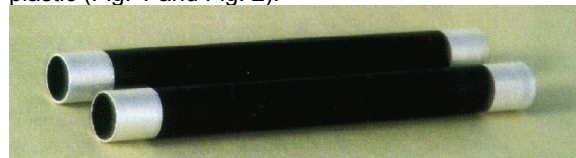
Fig.2. Current leads made of BSCCO tubes [5]
