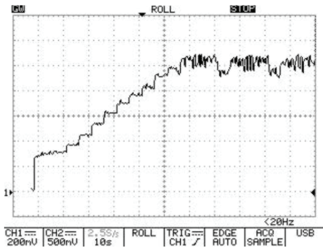
Fig. 13. The value of average current drawn by the transmitter in the process of tuning the output frequency of the inverter to the mechanical resonance frequency
