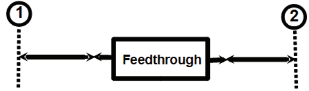
Fig. 2. The path inserted between the antenna and the receiver by measurement of radiated disturbances.
