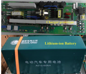
Fig.7 The charging system included charger prototype and lithium-ion battery pack for EV
