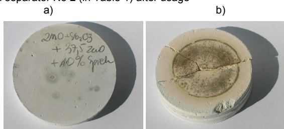
Fig. 3. The views of separator No 3 (in Table 1) a/ before and b/ after usage
