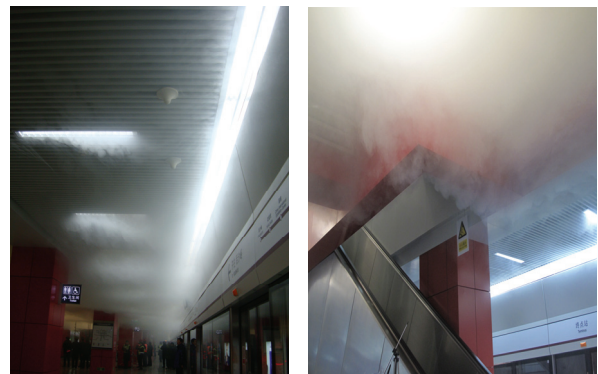
Fig. 13. Smoke accumulation on both sides of platform
