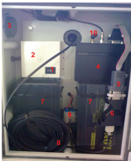
Fig. 5. Fiber glass box with the system hardware 1 - GSM/GPRS-GPS module on/off switch; 2 - Electric wiring box; 3 - GPS antenna; 4 - GSM/GPRS-GPS module; 5 - Cross RS232-RS232 cable; 6 - Optical-RS232 converter; 7 - 12V 7,2Ah battery; 8 - Fiber optic cable; 9 - Batteries terminal connection; 10 - GSM/GPRS antenna.
