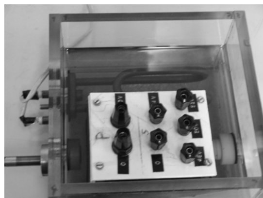
Fig.4 Test transformer 60 VA, 220/52 V - immersed in tank with transformer oil and heating apparatus
