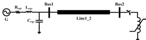
Fig. 1. Sample system for shunt reactor energization study. G: generator,  $R_{eqv}$ : equivalent resistance,  $L_{eqv}$ : equivalent inductance, and  $C_{eqv}$ : equivalent capacitance.
