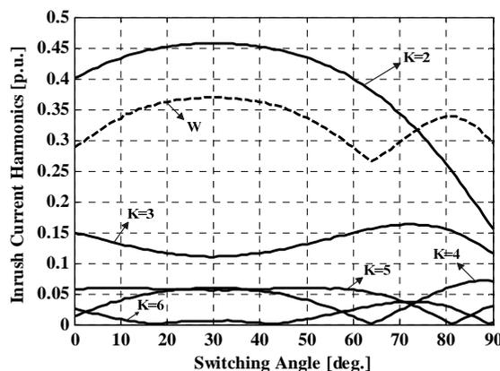
Fig. 3. Changes of harmonic currents and  $W$  index with respect to the switching angle.
