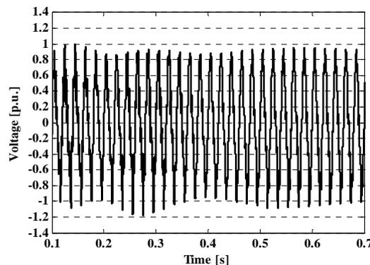
Fig. 4. Voltage at bus 2 after switching of shunt reactor for best switching condition.
